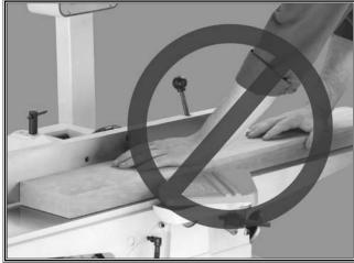
Figure 2. Never surface plane without push blocks!
